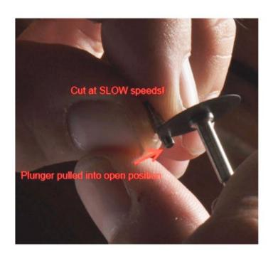
To shorten the attachment, pull the plunger into an open position and cut the plunger and housing together with a diamond disk.
