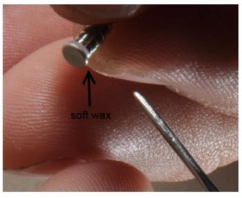
Before placing the attachment back into the access hole, with the attachment in a closed position, carefully seal the exit point of the plunger and housing with soft wax.
