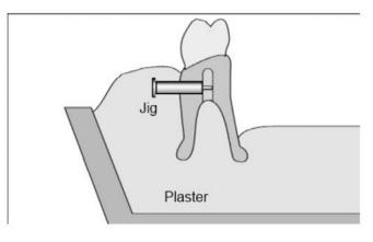
Wax-up completely around the processing jigs. Flask the completed set-up, making sure that the processing jig is indexed in plaster, and boil out.
