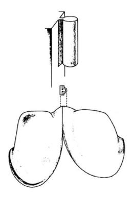
The Splintastik is an inexpensive and easy to use rod and tube attachment for non-parallel anterior abutments and segmented bridgework.
