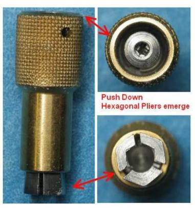
• Insert the sphere into the tool. The sphere will bypass the "loose" hexagonal pliers. Make sure that the hexagonal pliers are correctly oriented around the hex underneath the sphere.
